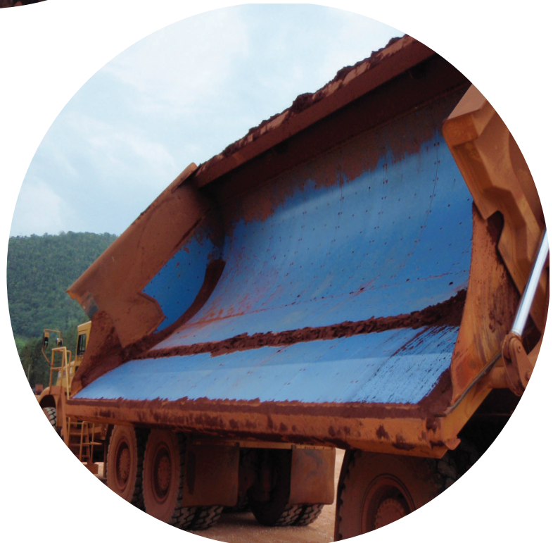
Side tipper truck tray after installation of Matrox lining
