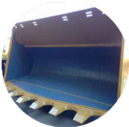
Loader bucket lined with Matrox Classic
