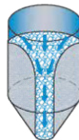
Funnel Flow: The flowing material (blue) is forming a funnel, while the rest (grey) is sticking to the walls of the bin.
