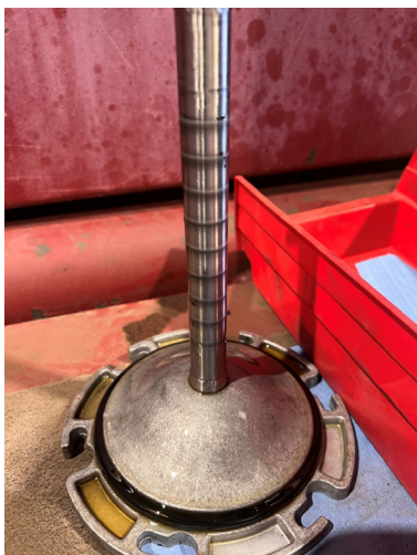
Figure 5: OEI custom fabricated Magnetic filter cap, with wear particles
