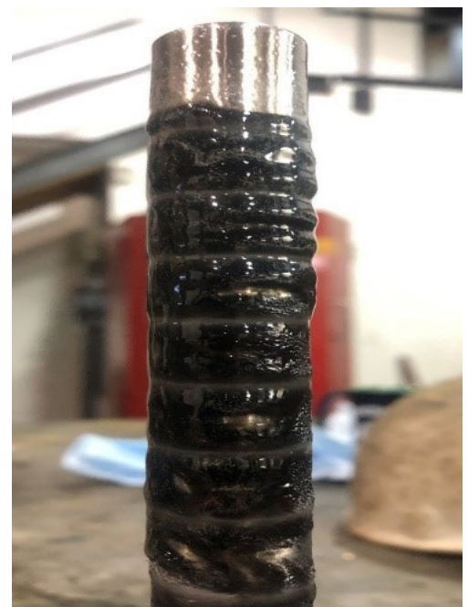
Figure 4: Contamination from the wet brake circuit captured by OEI Magnetic Y-Strainer
