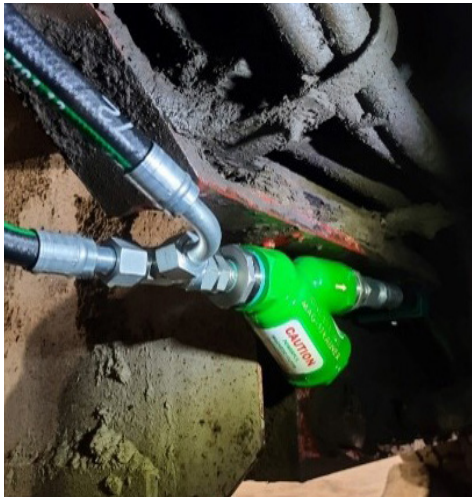
Figure 1: OEI's Magnetic Y Strainer attached to wet brake circuit.
