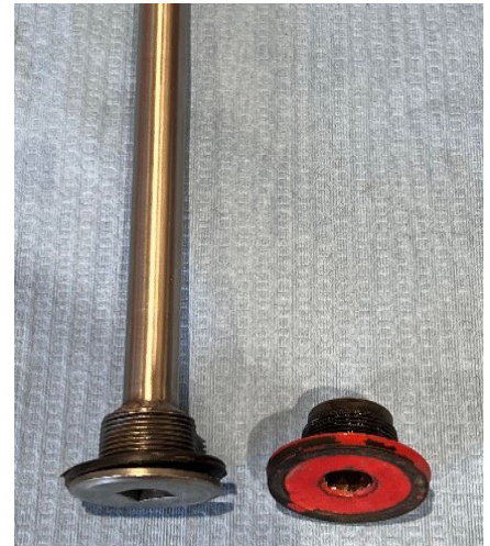
Figure 3: OEI Magnetic drain plug installed within the machine
