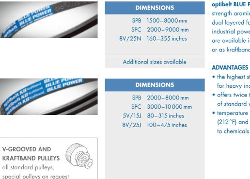
optibelt BLUE POWER's high tensile strength aramid cord and durable dual layered fabric wrap are ideal for industrial power applications. They are available individually, in sets, or as kraftbands.
