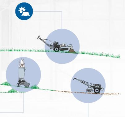
Garden shredders are used to shred or chip large volumes of any type of garden waste, hedge clippings. With the right power behind the shredder, almost anything can be shredded for using as mulch.
