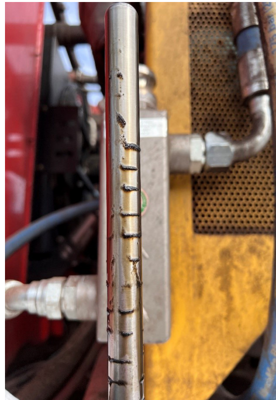
Figure 2: Wear contamination captured by the Magnetic Filter y-strainer over 500 hours, post traditional filtration.
