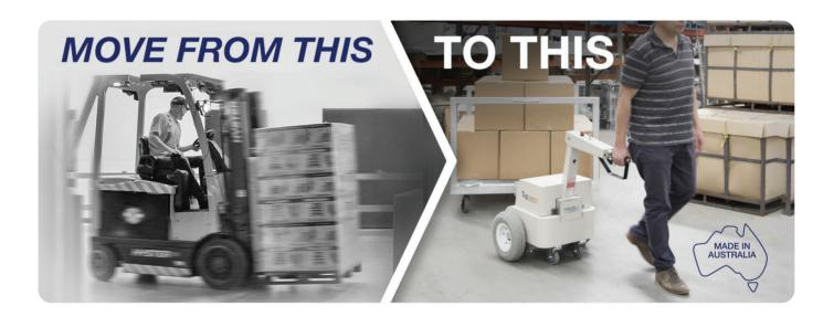
The powered tug's "front of load" ergonomic design ensures the operator maintains a "natural" walking position with maximum forward vision to avoid the risk of collisions.
