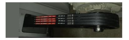
**Application:** Blower **Motor:** 75kW, 1450 rpm **Belt:** SPB 4750 RP
