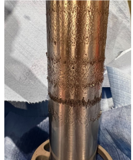
Figure 3: Picture of OEI magnetic scrubber element with captured contamination from diesel.
