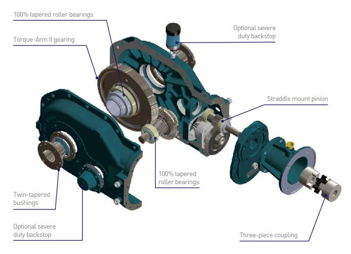
The Motorized Torque Arm II (MTA) is easy to install and built to last. It is a right angle, beltless direct-drive solution. This heavy-duty gear reducer is designed to deliver industry-leading performance in some of the most demanding applications.
