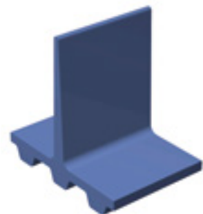
Figure 6.5.5: Triangular cleat with rounded head
